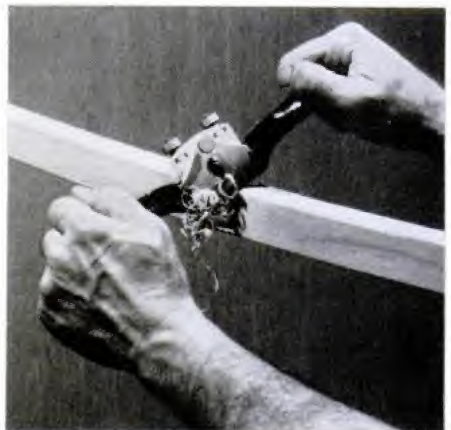
USE A SPOKESHAVE to round off the 1/8-in. plywood facing that must be added to one side of frame
